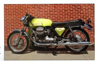
Italian hot-rod: Moto Guzzi shed its stodgy image in the early 1970s with its V7 Sport, combining the company's "sideways" V-twin with sport-style low bars and a four-leading-shoe drum brake.
